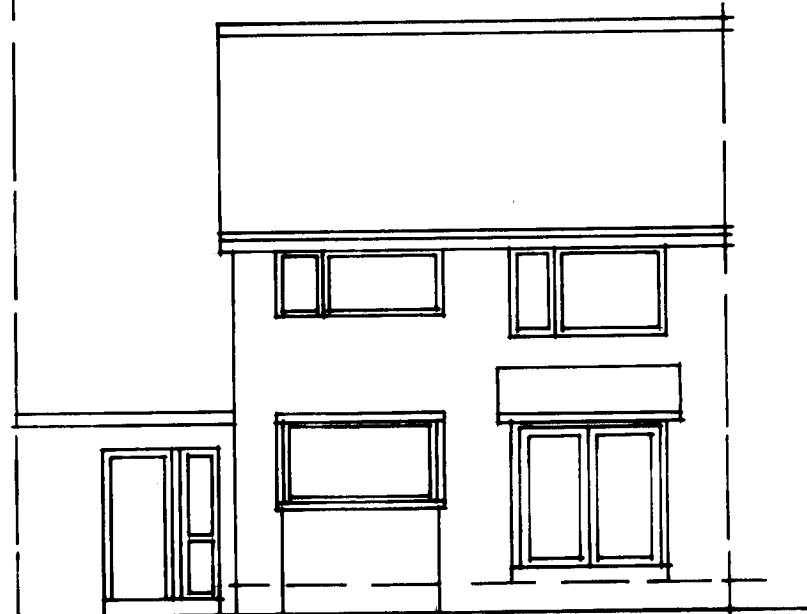
EXISTING REAR ELEVATION 1:100
